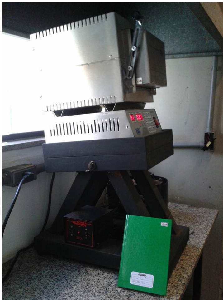
Figure A.2: Rocking furnace.
