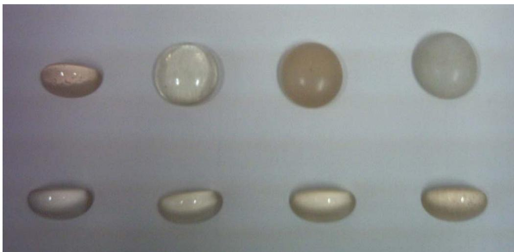
Figura 5.5 Amostras do vidro LSCAS co-dopadas com  $\text{Yb}^{3+}$  e  $\text{Ho}^{3+}$ .
